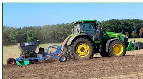
Soil 3 technique, strip-wise loosening and compost injection, in action at Klein Altendorf
